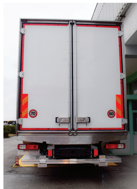
Unitrans "VR"-Series rear frame in stainless steel, thickness 4 mm
